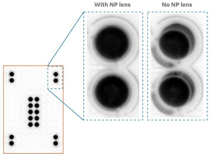
**Fig 14.** A chemiluminescent solution (ECL Select, 100  $\mu$ L per well) in a transparent 96-well plate (Corning™) shows that the NP lens enables artifact-free imaging. Distortions and obscured imaging, and subsequently higher variation in the analysis, is evident in corner wells without the NP lens.
