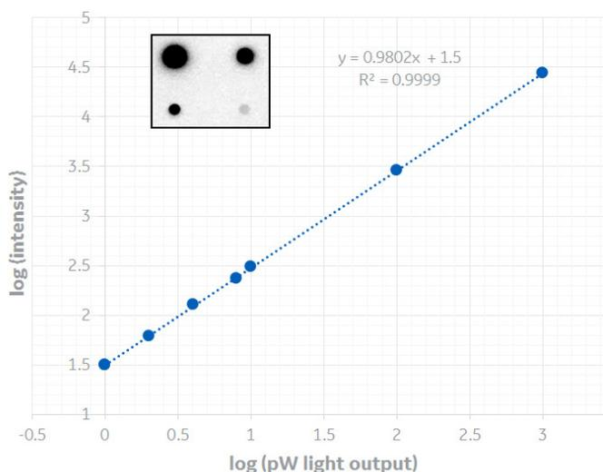
**Fig 17.** Amersham ImageQuant 800 imager exhibits excellent linear dynamic range. In this example, imaging of a calibrated luminescence plate in lower tray position, which emitted light power in the range 1 pW to 1 nW, showed linear response in recorded signal over the entire dynamic range. The inset image shows the 1 pW, 10 pW, 100 pW, and 1 nW light diodes (2, 4, and 8 pW not shown).
