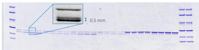
**Fig 22.** Colorimetric imaging with Amersham ImageQuant 800 imager results in high-resolution images for the most demanding applications. The zoom in of the Coomassie stained gels shows that it is possible to resolve bands on a gel which are only 0.5 mm apart. To be able to differentiate these bands was critical for research on self-cleaving tags.
