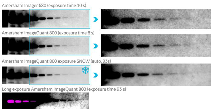
**Fig 9.** Intelligent SNOW detection algorithm in chemiluminescence mode dramatically improved the dynamic range and image quality by imaging weak bands without saturation of high intensity bands, enabling accurate quantitation of both strong and weak bands
