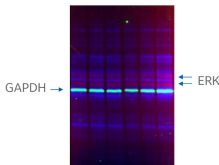
**Fig 19.** Three-color overlay image of Western blot nitrocellulose membrane. Target ERK proteins were detected using an IR long (red) LED-filter combination and GAPDH detection used an IR short channel (green). Lysates were pre-labeled with Cy3 (blue).
